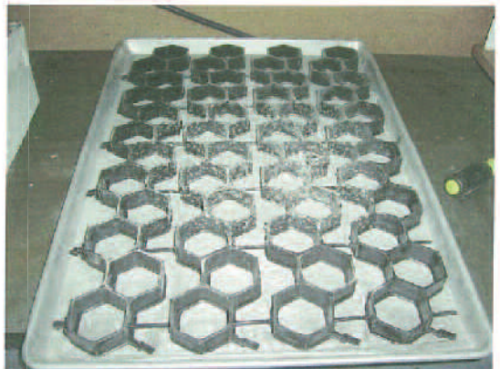
Photo No.4: After Test NDS EZ Roll Gravel Paver (12-In.x 12-In. Compression Loading Plate: Aggregate @ Flushed) (Proof Load = 500,000Lbs.)
