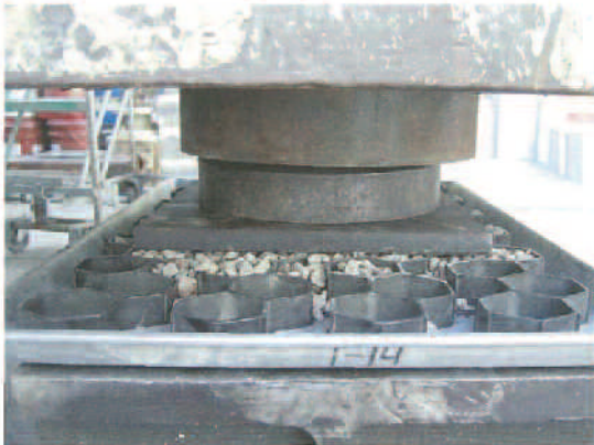
Photo No.2: Test Set-up NDS EZ Roll Gravel Paver (12-In.x 12-In. Compression Loading Plate: Aggregate @ Flushed) (Proof load = 500,000Lbs.)
